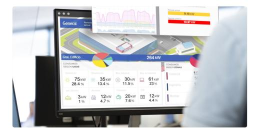
By installing power analyzers, you can have real-time information on electrical parameters, such as voltage, current and harmonics. You can use all this information to determine the power quality and to know where, when and how much energy the different loads in your installation consume.
